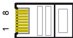
Abb.2 Contact/pin assignments of RJ45 plug
